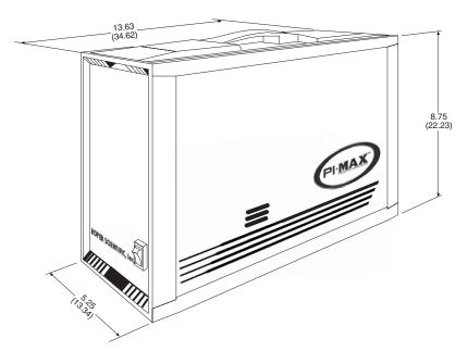
Figure 41. ST-133A Controller Dimensions
